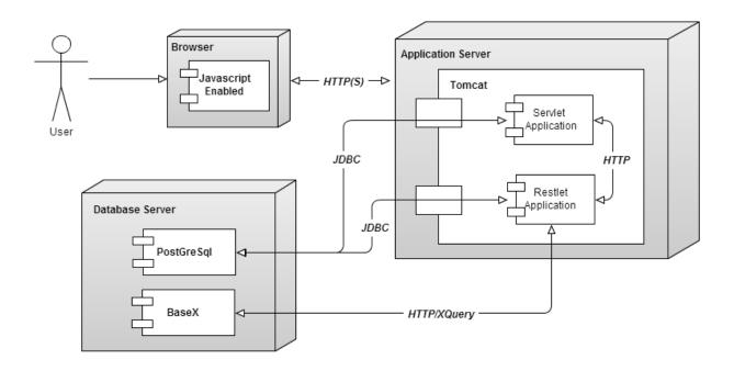
The diagram above shows a modular representation of the system design. Each box represents a logical tier (including client, application, and database). Within each box resides a component which is connected to one or more dependencies by the protocol indicated.
